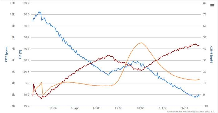
Figure 3: Graph of ethylene (orange), oxygen concentration (blue) and CO2 (red). This information comes directly and real time from the userportal. The ethylene production of the crop is directly related with the day- and night rhythm of the respiration which comes from the photosynthesis process.
